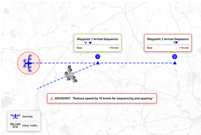
Notional user view of SkyGrid's Flow Management service, showing a speed change advisory to maintain in-trail separation between aircraft.
