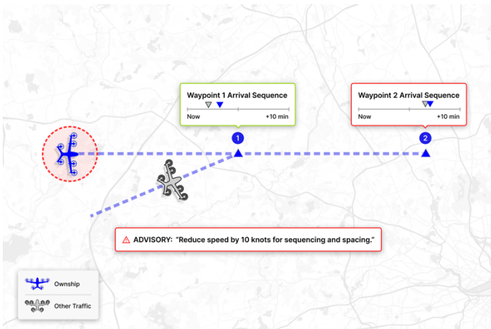
Notional operator view of SkyGrid's Flow Management service, showing a speed change advisory to maintain in-trail separation between aircraft.
