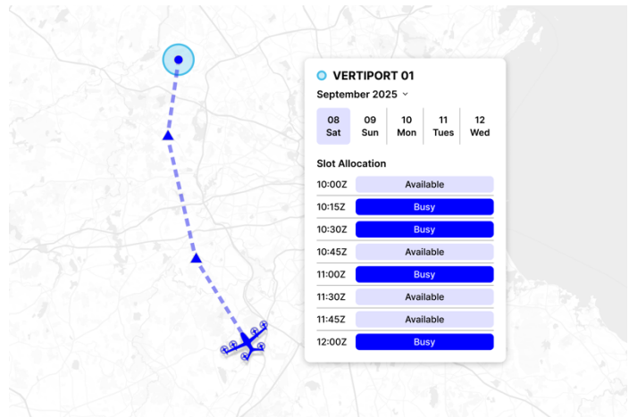
Notional operator view of SkyGrid's Resource Status and Capacity Data service, showing available slots for arrival and handling at a vertiport.
