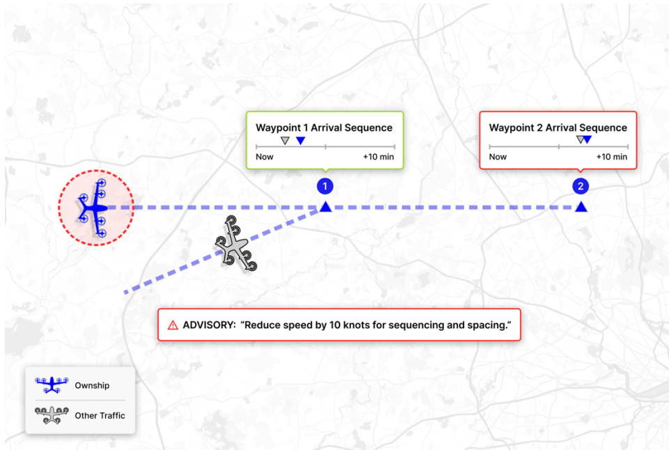
Figure 16. Notional operator view of SkyGrid's Flow Management service, showing a speed change advisory to maintain in-trail separation between aircraft.
